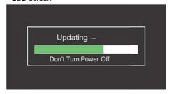
(4) After update is completed, it is displayed on LCD as "Complete". (Update time is about 3 minutes.) SLOT A LED and SLOT B LED carry out green blink simultaneously slowly.
